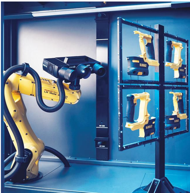
Automated scanning of plastic parts with the ATOS scanner. (Provided by Capture 3D)
