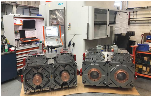
Moldmaker Moulexpert chose the Mikron MILL P 800 U ST to achieve tolerances in the range of 5 \mu m that are needed to machine thin-wall molds for the packaging industry. (Provided by Moulexpert and GF Machining Solutions)
